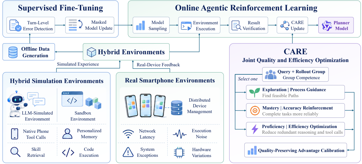
Figure 4: Training framework for the Planner Model in Qwen-Planner-Agent. Supervised fine-tuning with turn-level error detection and loss masking establishes a planning-oriented cold-start policy, followed by online agentic reinforcement learning in hybrid environments combining LLM simulation, programmatic sandboxes, and selected real-device interaction. Within the RL stage, CARE (Competence-Aware Reward-and-Advantage Engineering) selects process guidance, accuracy reinforcement, or efficiency optimization according to each trajectory group’s competence. Quality-preserving advantage calibration limits the amplification of small efficiency differences, promoting efficient reasoning and tool use while retaining verified task success as the primary objective.
